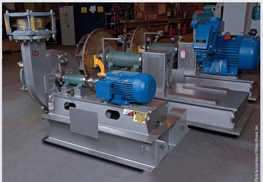
Blower for a pressurized dust collection system within a petrochemical reactor
