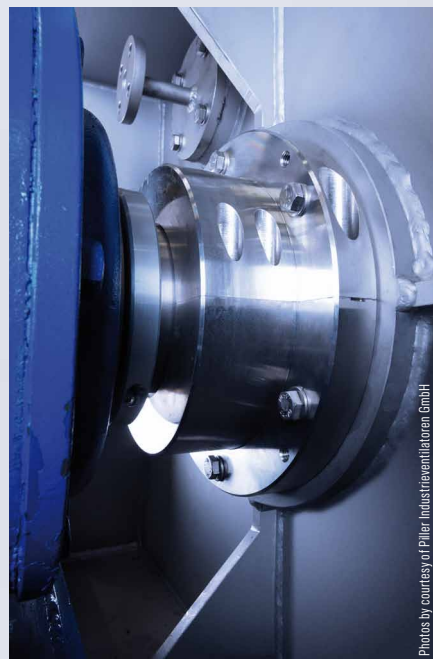
Carbon floating ring seal Espey WD500, type WDSA
