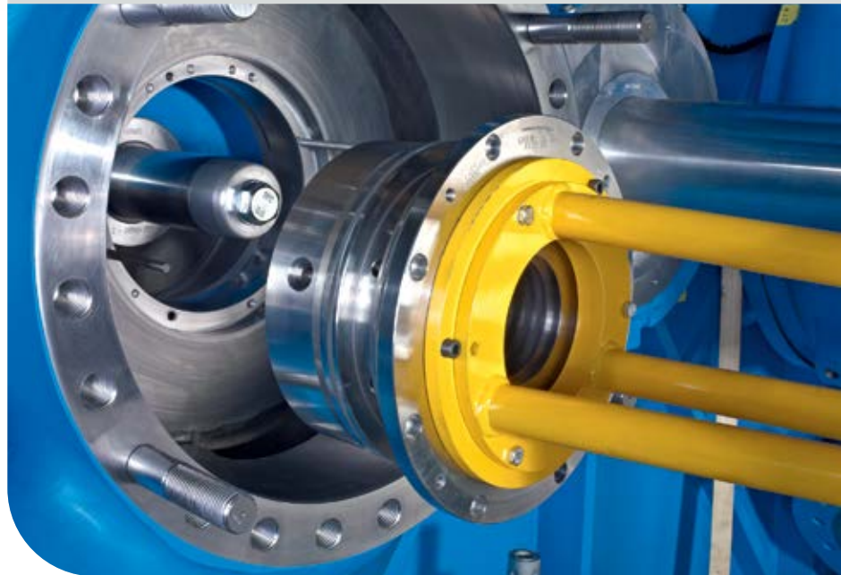
Installation of Espey WKA802 into a gear compressor
