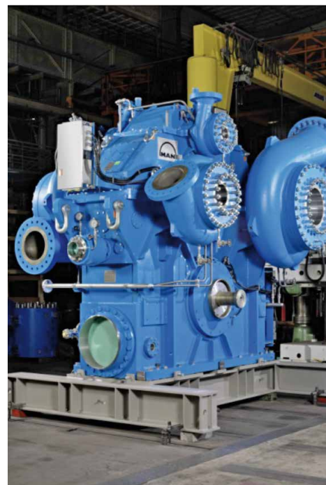
Multi-stage gear compressor
